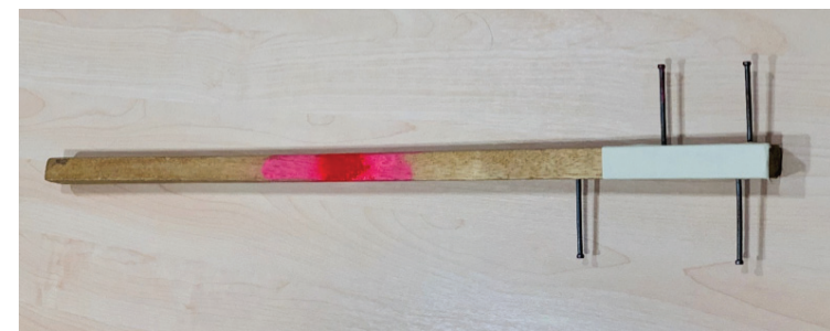
A simple measuring guide for estimating stem diameter range
